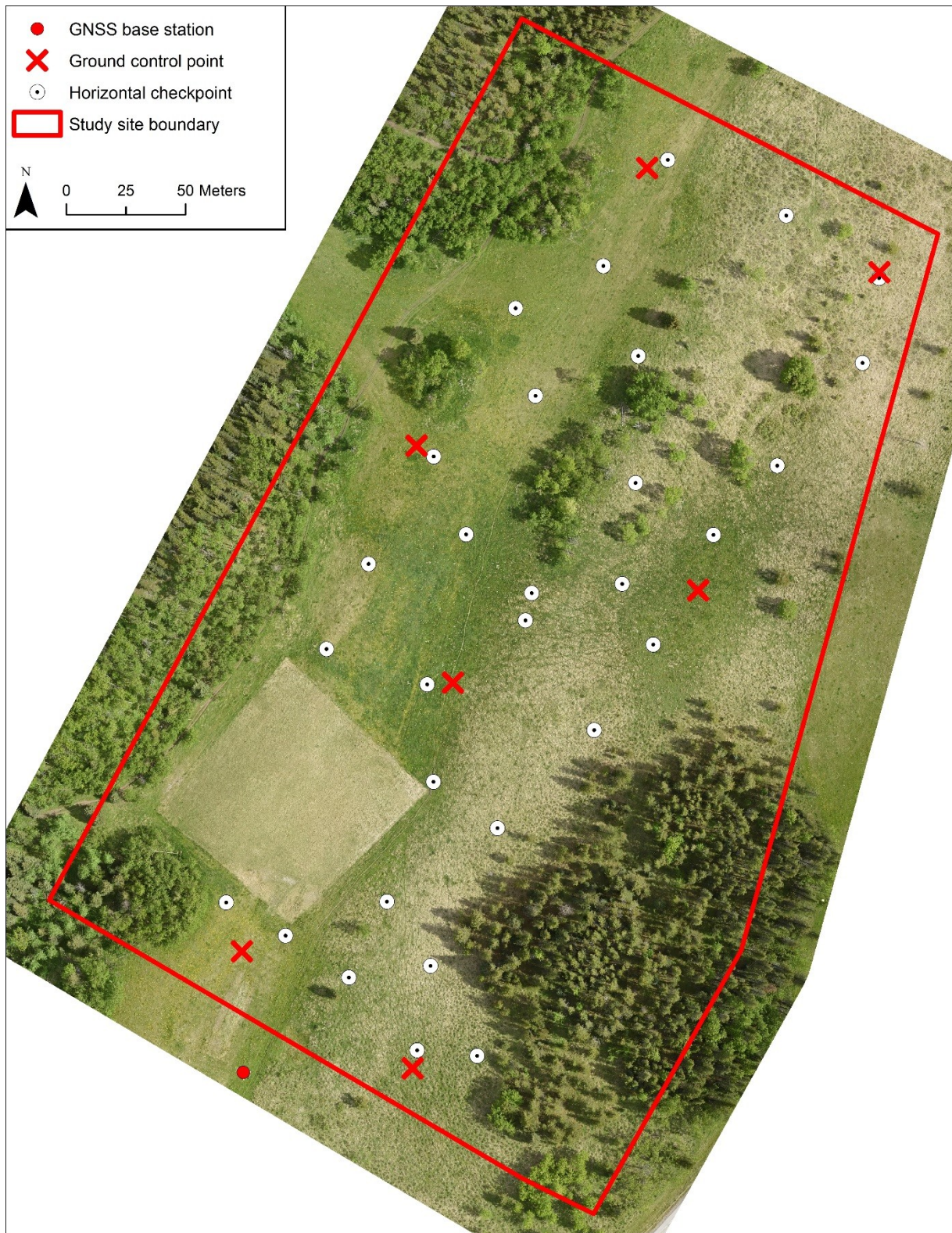
Figure 2.4 Location of RTK GNSS base station, ground control points, and horizontal checkpoints.
